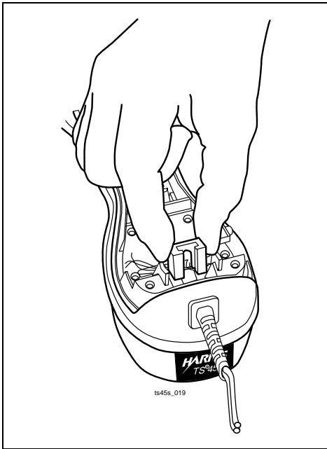
Figure 9. Removal/Installation of the Plastic Clip
