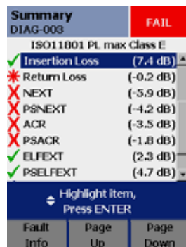
Figure 4: Upon completion of an Autotest, the tester’s screen shows the list of test parameters executed for the selected test standard. Test parameters marked with the red X fail. The tester also displays the worst-case margin for each parameter in parentheses at the right edge of the screen.
